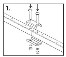
Join the 2 pieces of boom together using the joining plate, M5 x 20mm screws M5 nuts and 5mm Shake Proof Washers.
