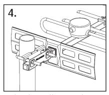
Attach aerial to a suitable mast using the supplied Mast Clamp. (Note: Mast not supplied).
