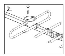
Screw on firmly the Dipole to the Boom.
