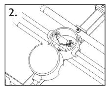
Loosen the screws on the 2 terminals in the Dipole. Feed the inner core to one of the terminals and the twisted braid into the other. Tighten screws and close Dipole Cap.
