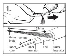
Thread coaxial cable through Dipole Cap. Strip away 25mm of outer insulator. Gather outer braid strands and twist together. Remove 10mm of inner insulation around inner core.
