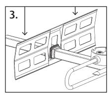
Slide on and firmly push down the Reflector onto the groove of the Reflector Bung.
