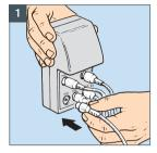
Connect the coaxial lead from your TV or Radio and aerial down lead (single or diplexed) into the front section of the booster.
